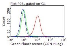
HEK293T cells transfected with either [RC209954] overexpress plasmid (Red), compared to an IgG isotype control, (Green) or empty vector control plasmid (Blue) were immunostained by anti-ERBB3 antibody ([TA803827]), and then analyzed by flow cytometry (1:100).
