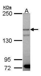
Sample (30 ug of whole cell lysate). A: A431. 5% SDS PAGE. TA308734 diluted at 1:1000.
