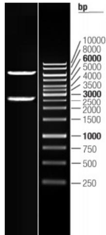
Double digestion of RC213837L1 using SgfI and MluI
