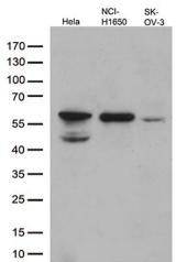
Western blot analysis of extracts (35ug) from 3 different cell lines by using anti-KRT7 monoclonal antibody (1:500).
