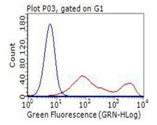
HEK293T cells transfected with either [RC219458] overexpress plasmid (Red) or empty vector control plasmid (Blue) were immunostained by anti-BTLA antibody ([TA505536]), and then analyzed by flow cytometry (1:500).
