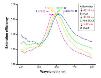
Figure from citation: LSPR spectra for processing steps of immobilization and detection of 100 pM SCCa. (A) Bare silver nanochip, ?max =573.92 nm. (B) Modification of 1 mM MUA, ?max =589.1 nm. (C) Incubation with 10 ug/mL monoclonal anti-SCCa, ?max =602.38 nm. (D) Detection of 100 pm SCCa, ?max =612.15 nm.Note: All spectra were collected at room temperature in air.Abbreviations: LSPR, localized surface plasmon resonance; MUA, 11-mercaptoundecanoic acid; View Citation
